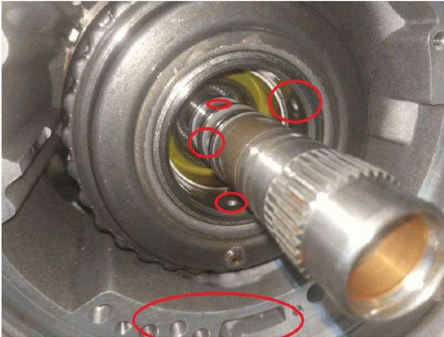
To travel from the hydraulic distributor to the piston clutch, the fluid passes through a series of holes drilled in the transmission housing and in pipes incorporated in the central hub, before joining the rotating drum containing the annular piston.
