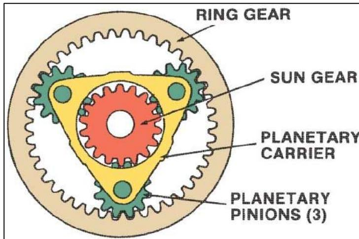
This is the actual heart of the BVA. It provides 4 forward gears and one reverse. It consists of a set of gears, which blocks or releases that depending on the desired speed.
