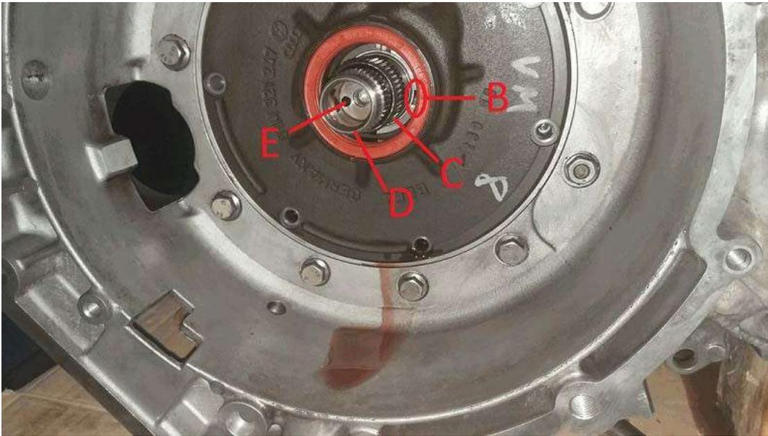
External gear grooves (C) are fixed. The internal grooves (D) correspond to the automatic gearbox the input shaft which transfers the engine's torque.
