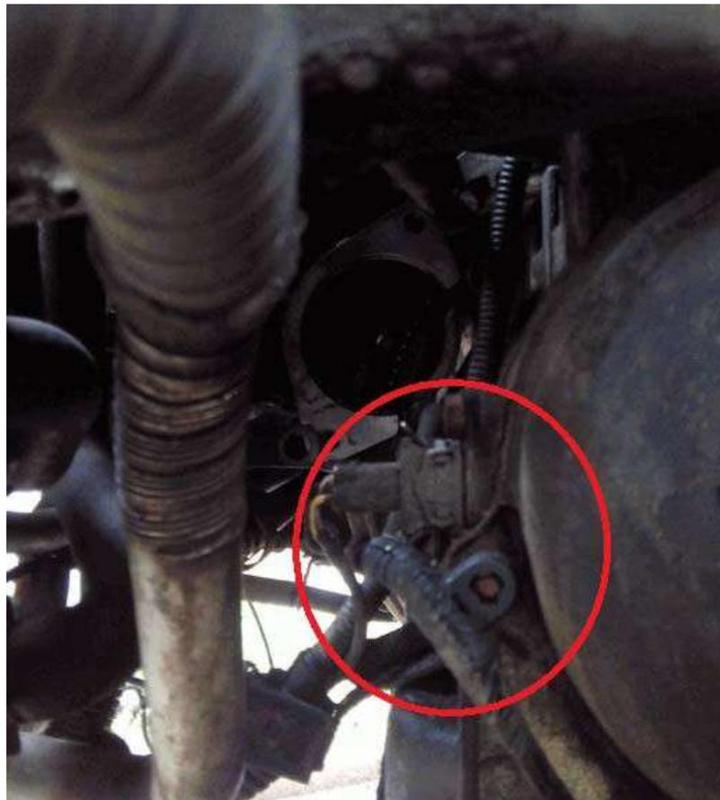
The BVA has its own electric pulse which links the transmission's computer (TCM) to hydraulic distributor.
