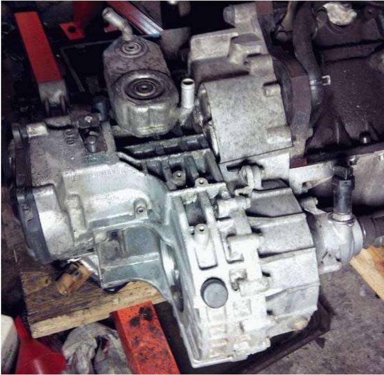
Cousin of Renault AD4, the AG4 automatic transmission, which has equipped many models of the VAG group (including the Transporter) until 2003 is a French design!
