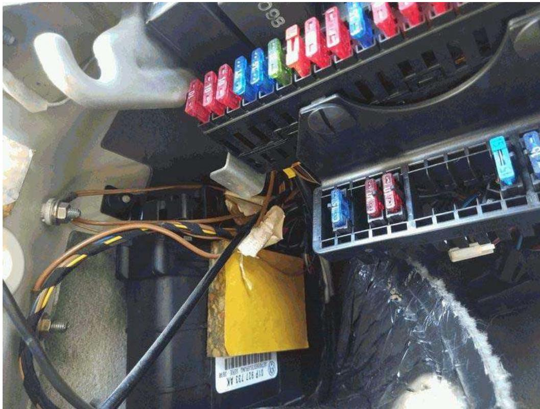
Called in English "Transmission Control Module" or TCM. It can be found in the passenger cabin, on the right side on the first-generation models, or on the left side, close to the inner wheel housing, on newer models.
