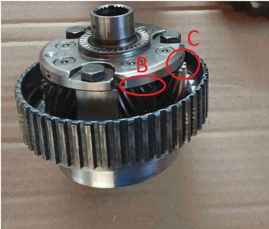
At first glance, all 6 satellites side by side gears may appear "identical", but closer look reveals that only those marked (C), driven by the large sun gear are linked with the output ring of the planetary gear train.
