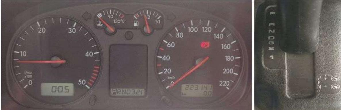
Another difference, audible this one, is the frequent printing of "skating-slipping" because the engine speed is not proportional to that of the wheels. This difference is due to the converter slip.
