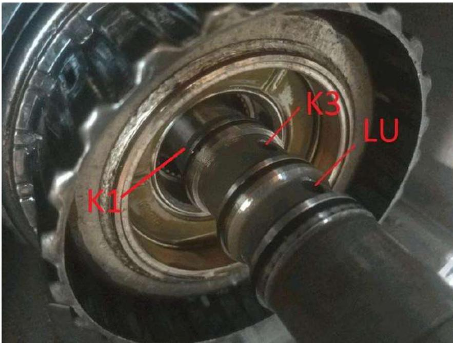
The axis main BVA comprises a series of segments, annular metal seals (oil sealing rings), which realize a rotating seal.
