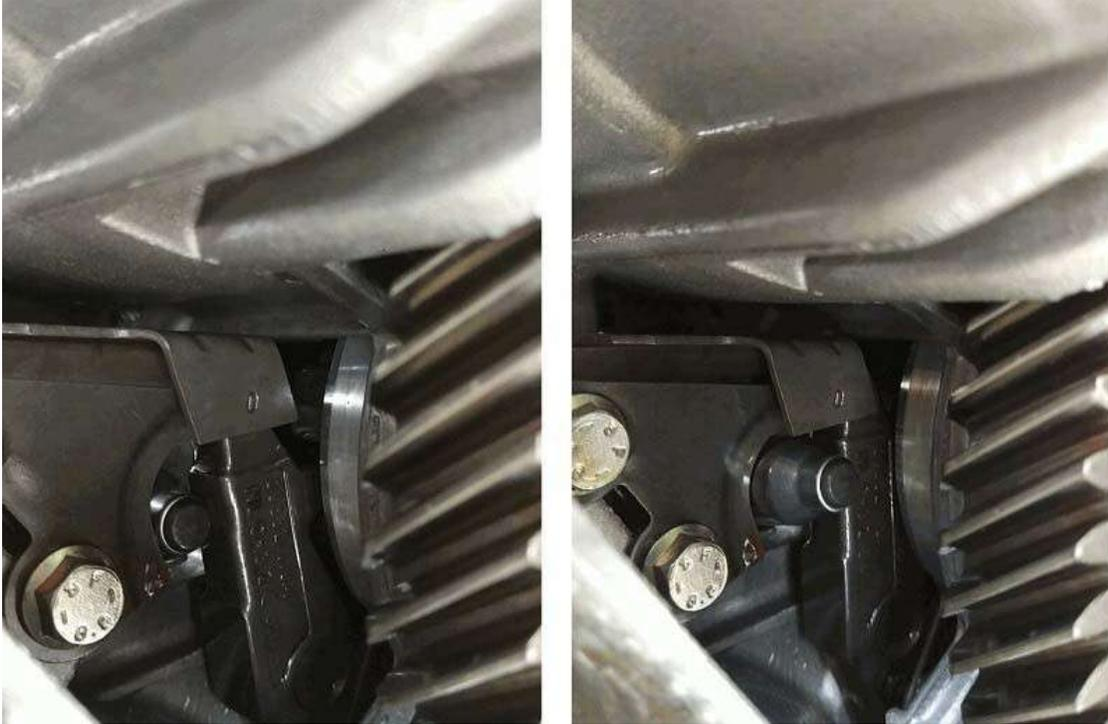
We have seen that in Parking mode, the engine and the wheels were never connected, so it is impossible to put a gear "engagement" to block the vehicle.
