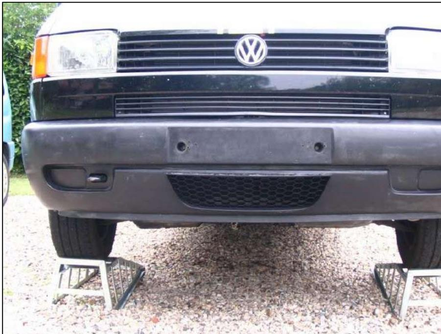
Cooling of the BVA may improve by using the same techniques used by VW Syncro: Air vent opening in the lower bumper section and cutting an opening in the underbody steel pan.
