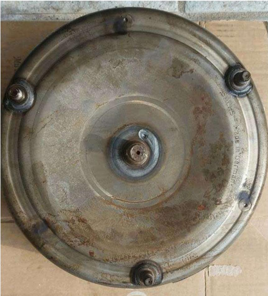
The torque converter (or TC) as seen on the engine side.
