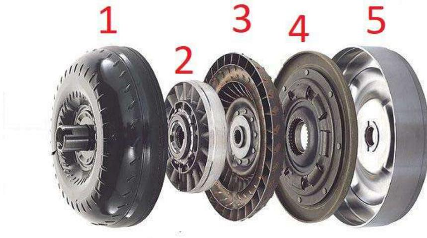
The "Bell" (1) is welded to the converter bottom (5) itself screwed to the flywheel, and thus rotates continuously. It is connected by a set of "fingers" to the oil pump of the BVA.
