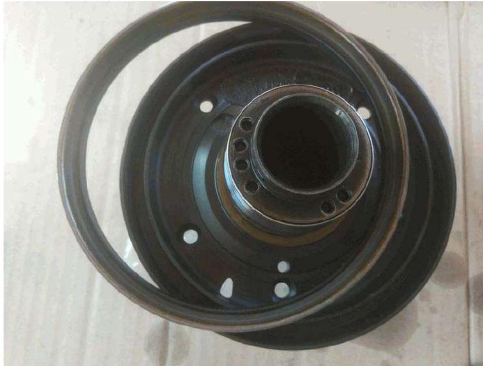
On some types of BVA (AL4), the brakes are strips that rub on drums. On AG4 by contrast, the brakes are much like clutches. Their discs and pistons have the same shape but have larger diameter, because they surround the rotating clutches.
