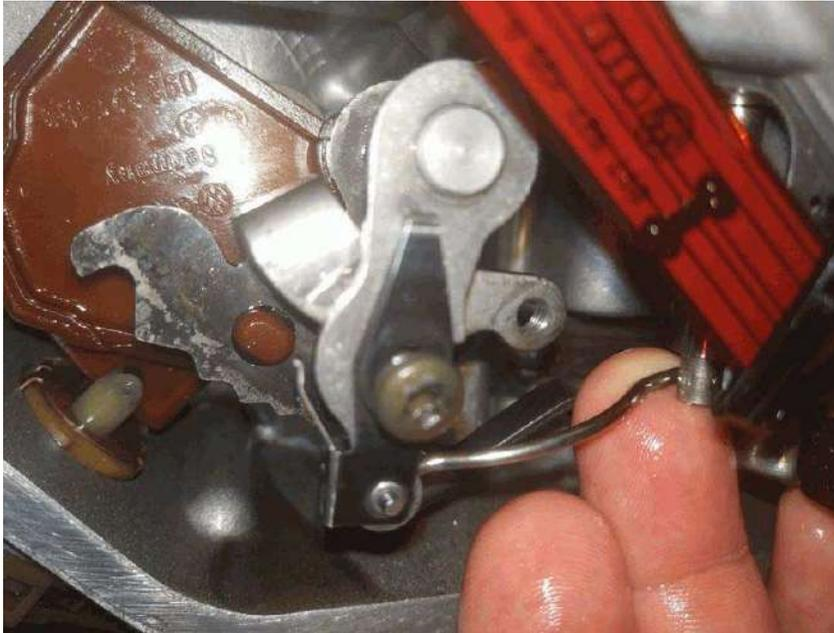
Controlled by a set of cams and feelers, the CMF (Multifunction Switch) indicates the position of the selector to the computer.
