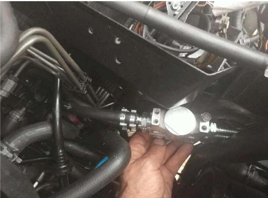
The radiator works so well that the oil is likely to remain at a temperature lower than what's recommended. For me (intentionally oversized radiator) on the highway at 130 km/h ATF remained at 70°C (158F) with 30°C ambient temperature. (86F)
