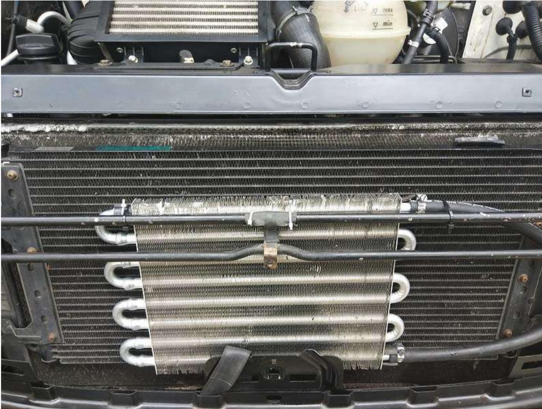
Replacing the original oil/water exchanger with a beefier one.
