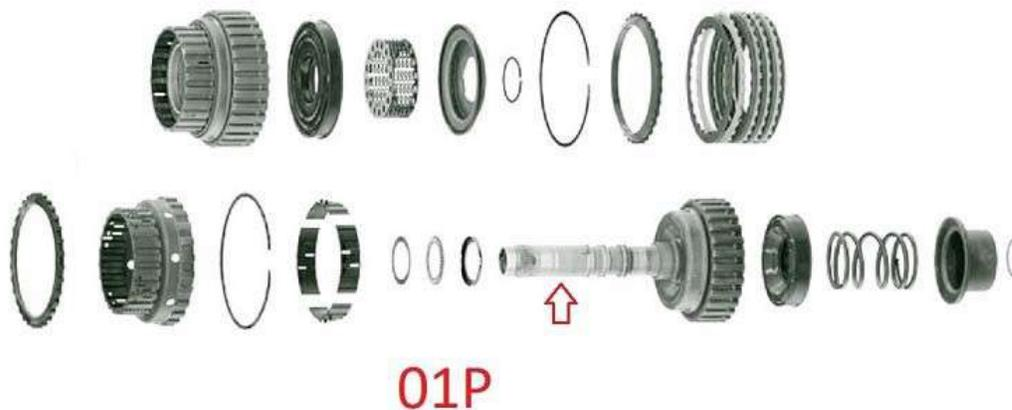
The main difference is that the 095 / 01M features two concentric axes, as of the 098 / 01P contains only one. The shape or the thickness of certain parts also varies: trays, springs ...
