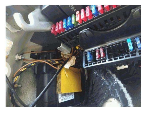
Called in English ''Transmission Control Module'' or TCM. It can be found in the passenger cabin, on the right side on the first-generation models, or on the left side, close to the inner wheel housing, on newer models.
