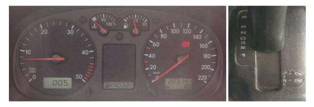
Another difference, audible this one, is the frequent printing of "skating-slipping" because the engine speed is not proportional to that of the wheels. This difference is due to the converter slip.
