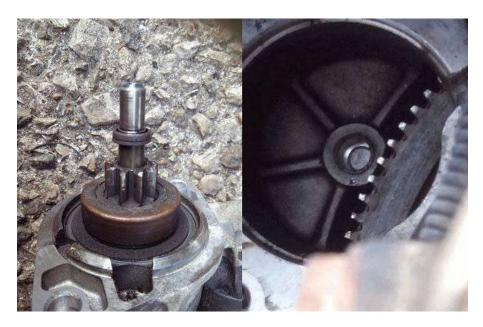
It is specific to the BVA: two fastening screws as of 3 for the BVManual. The bearing bronze of the output shaft is lodge in the bell of the converter, and not in the starter. When replacing a starter, it may be essential to change too!
