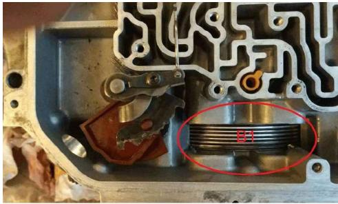
injecting compressed air in the little yellow tube.
