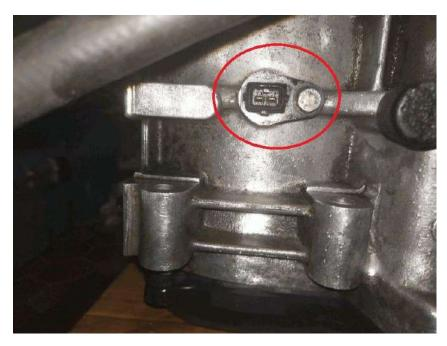
The BVA houses 2 or 3 magnetic reluctance sensors, robust and reliable (similar to some present on ABS rings)
