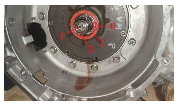
External gear grooves (C) are fixed. The internal grooves (D) correspond to the automatic gearbox the input shaft which transfers the engine's torque.
