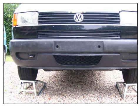
Cooling of the BVA may improve by using the same techniques used by VW Syncro: Air vent opening in the lower bumper section and cutting an opening in the underbody steel pan.
