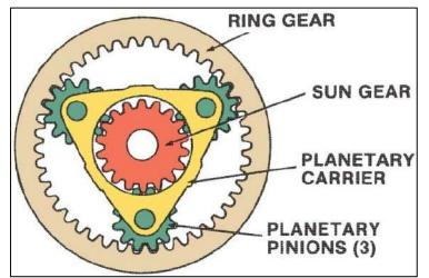
This is the actual heart of the BVA. It provides 4 forward gears and one reverse. It consists of a set of gears, which blocks or releases that depending on the desired speed.
