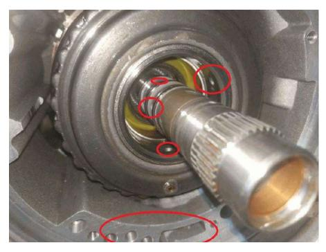
To travel from the hydraulic distributor to the piston clutch, the fluid passes through a series of holes drilled in the transmission housing and in pipes incorporated in the central hub, before joining the rotating drum containing the annular piston.
