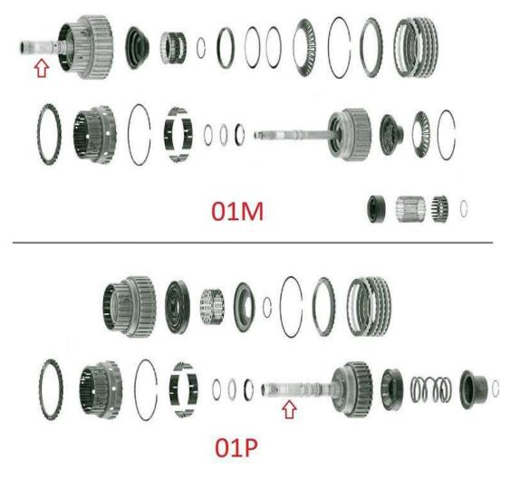
The main difference is that the 095 / 01M features two concentric axes, as of the 098 / 01P contains only one. The shape or the thickness of certain parts also varies: trays, springs ...
