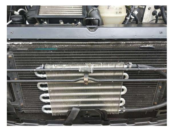
Replacing the original oil/water exchanger with a beefier one.
