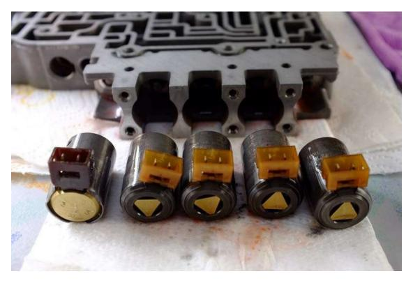
They're 7 solenoids all together. They're connected by a frangible web to a circular connector, ensuring the connection with the computer. Please note that this table also contains the temperature sensor. The web is permanently immersed in oil.
