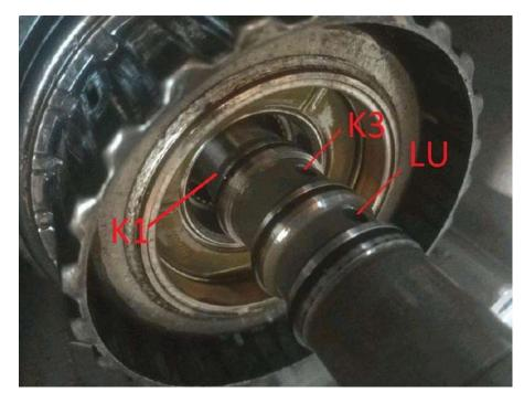
The axis main BVA comprises a series of segments, annular metal seals (oil sealing rings), which realize a rotating seal.
