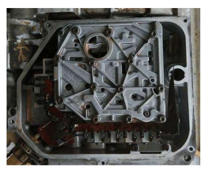
It incorporates driver commands and of the BVA computer sending the oil in the various corresponding circuits.
