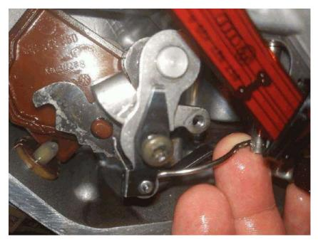
Controlled by a set of cams and feelers, the CMF (Multifunction Switch) indicates the position of the selector to the computer.
