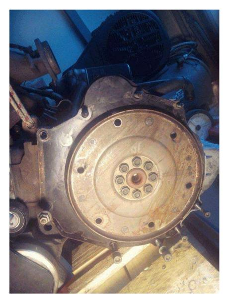
On every BVA, the flywheel is a simple plate of pressed sheet metal, perforated with holes through which grips with the converter.
