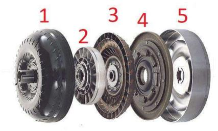
The "Bell" (1) is welded to the converter bottom (5) itself screwed to the flywheel, and thus rotates continuously. It is connected by a set of "fingers" to the oil pump of the BVA.
