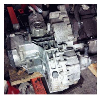
Cousin of Renault AD4, the AG4 automatic transmission, which has equipped many models of the VAG group (including the Transporter) until 2003 is a French design! The AD4 box was designed by the STA ("Société de Transmission Automatique"), whose factory are located in Ruitz, in the Pas-de-Calais.
