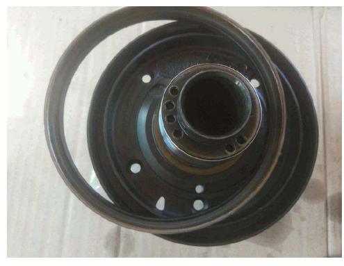
On some types of BVA (AL4), the brakes are strips that rub on drums. On AG4 by contrast, the brakes are much like clutches. Their discs and pistons have the same shape but have larger diameter, because they surround the rotating clutches.
